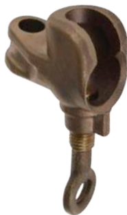
Ball Stud Ground Clamp accepts 30 mm Ball Studs Grade 5H Rated Catalog No. PSC6003494 Drilled for 5/8-11 UNC threaded ferrule
