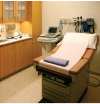
Patient beds in general care locations require a minimum of eight hospital grade receptacle outlets, single or duplex
